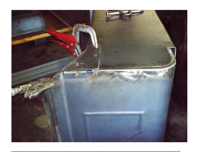
Step 6: Clamp bracket as shown. Weld or rivet at least one per flap. (4 points) Box should be really solid at this point.
